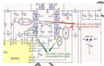
Figure 13 Schematic
